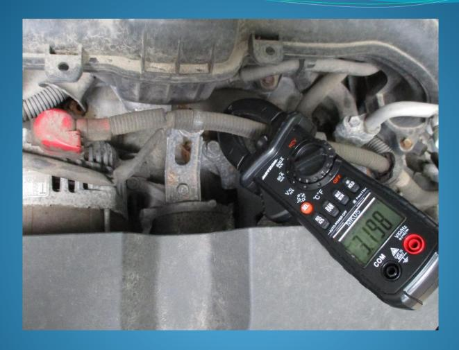
Engine warm, 750 rpm, alternator cable 3.0 amps, 30.0 mG. The alternator generated current travels through alternator cable to charging controller and then to the positive battery terminal. To complete the alternator circuit, the current leaves the negative battery terminal which is electrically connected to the metal car chassie. The current takes all paths available back to the alterator housing.
