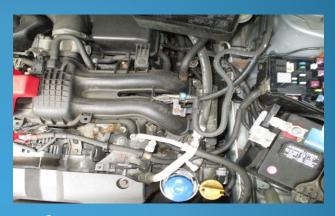
Testing the addition of grounding wires running next to alternator cable (between the alternator metal housing and the metal car chassie near the battery) as an additional path to complete the alternator circuit and lower Alternator cable net amps and total magnetic fields.
