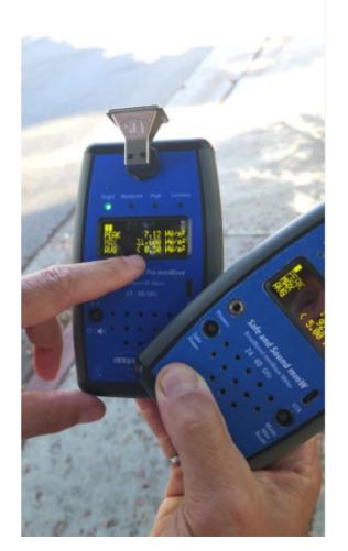
mmWave antenna and phone signal strengths, two mmWave RF meters with horn antennas, beam-form triggered by phone data usage
