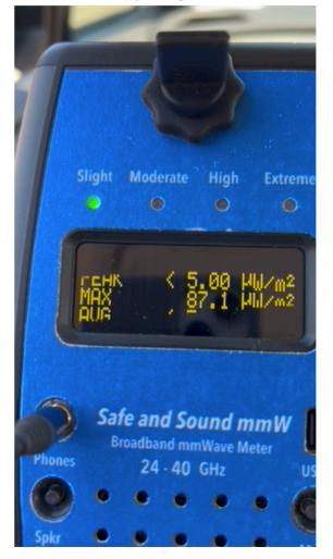
mmWave antenna signal strength closer with stub and horn antennas
