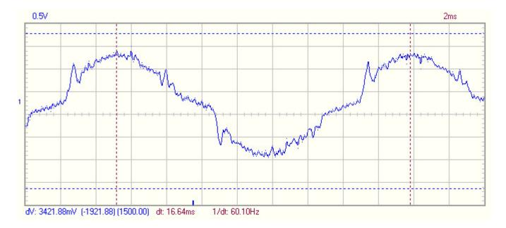
This could be assumed to be from the smart meter, however, the harmonic is not short or sharp with a fast slew rate like the harmonic shown in Rob States' image.
