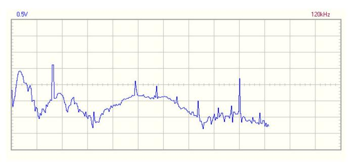
Here is the same analysis with a single Greenwave filter inserted, showing a clearing of the noise at many frequencies:
