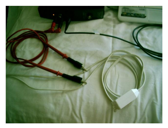
I found that it is important to connect the lead clipped to the hot wire of the extension cord into the red input of the Pomona connector, and that you connect the lead clipped to the neutral wire into the black input of the Pomona connector.
