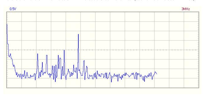
Here is the same analysis with a single Greenwave filter inserted, again showing significant clearing of most noise except for one spike at approximately 1.4MHz:
