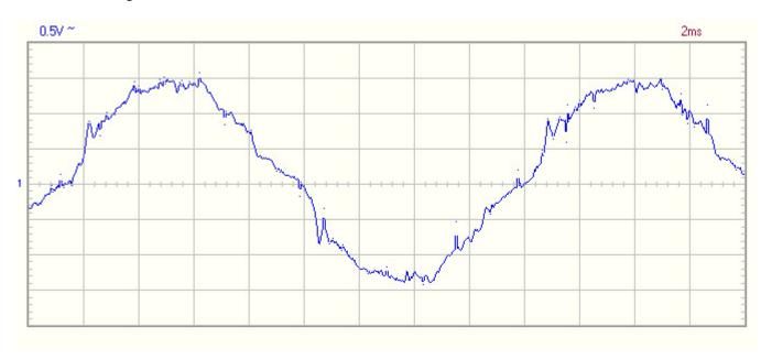
Note below that the fundamental frequency this time is 3 kHz and the height is less than half a Volt  $(0.47 \text{ Volt in } 320 \text{ microSeconds}, \text{ for a slew rate of only } 1,470 \text{ V/sec} - \text{see below for the significance of these numbers}):}$
