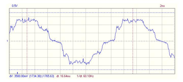
To once again demonstrate that the new protocol does demonstrate voltage harmonics when present, the following tracing shows the same circuit but this time with a dimmer switch turned on in an adjacent room. Notice the large, short, sharp repeating harmonics just before the height of each peak that measure almost 2 Volts high (almost four vertical squares at half a Volt per square).
