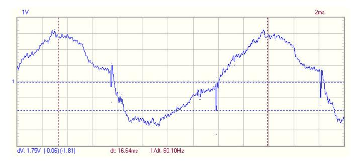
Here is the same waveform tracing taken at the same time of channel two by itself, showing the same recurring harmonic from the dimmer switch but without the 60 Hz sine waveform, which was flattened by the Stetzer attenuator:
