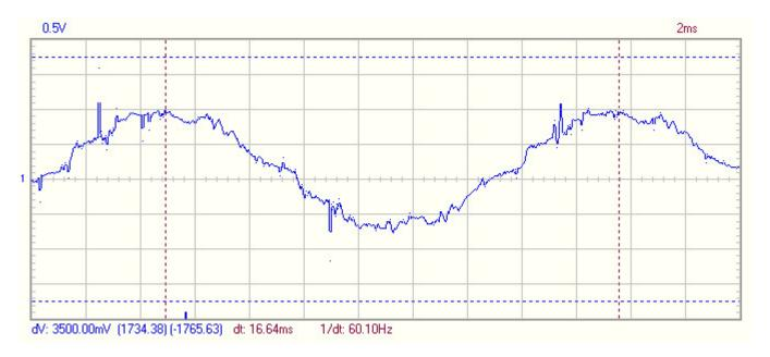
The tracing below is a closeup of the transient, which appears to have a fundamental frequency of 17 kHz and a size of 1.3 Volts in 60 microSeconds, for a slew rate of 21,600 V/Sec:
