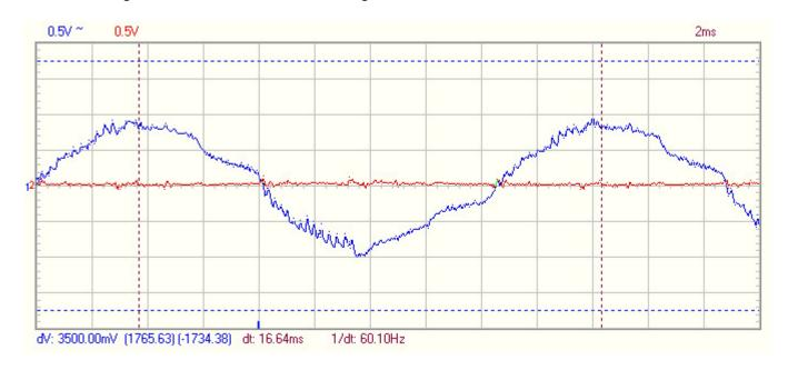
When I shut off all other circuits except the one that powered the outlet I was plugged into, both waveforms looked a little cleaner (less spikes, less saw-toothed appearance), however you can see that there is still a little roughness or electronic noise in the portion of each cycle leading to a peak, particularly the minus (downward) peak:
