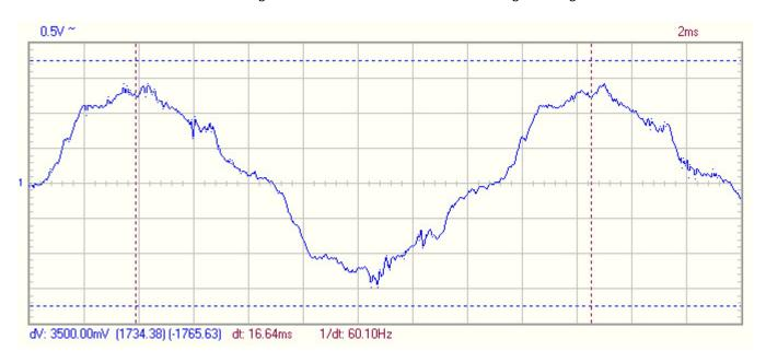
Again, there is no evidence of significant harmonic frequencies on the waveform tracing with the presence of the new digital meter.
