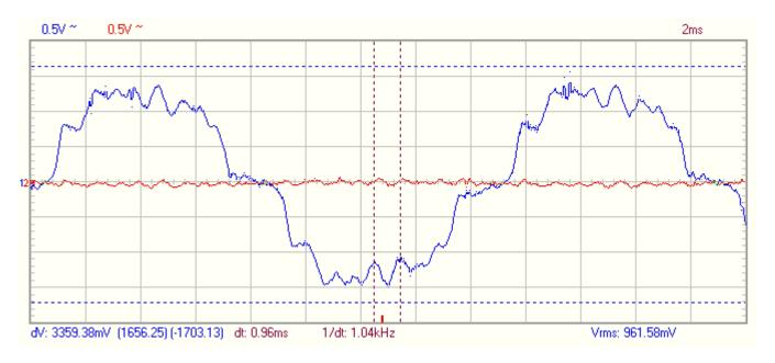
Compare this relatively clean oscilloscope tracing to the tracing below, this time with the inverters turned on. A higher frequency is superimposed upon the 60 Hz sine wave, as seen on both channel B connected to the circuit (red) and on channel A connected to the whip antenna in the air (blue):
