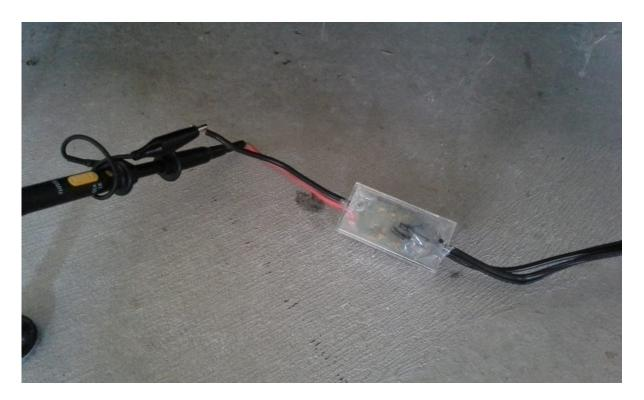
The wired lead is connected to the two wires of the Stetzer attenuator, which is plugged into an outlet:
