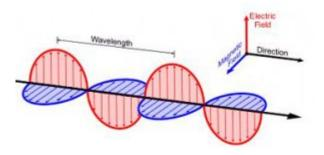
The following image, from <u>livescience.com</u>, shows this three-dimensional configuration where the electric and magnetic field components of electricity emit from a power line, circuit, cord or wireless transmitter at right angles to one another:
