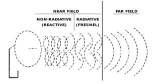
Thus, we recommend that anyone measuring smart meters with radio frequency detectors commonly available now should take their measurements at three feet and beyond for accuracy. This is because the electric field portion and the magnetic field portion of the transmission have not coalesced into a stable wave until they reach three wavelengths, which is the beginning of the far field. If you measure closer than three feet, you will get a reading, but it is not accurate.
